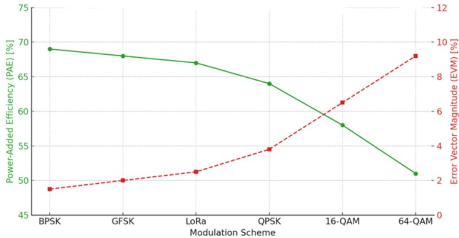
Figure 5. Efficiency vs. Linearity Trade-Off Across Modulation Schemes
