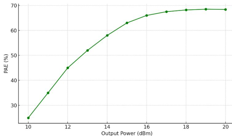
Figure 3. Power-Added Efficiency (PAE) vs Output Power
